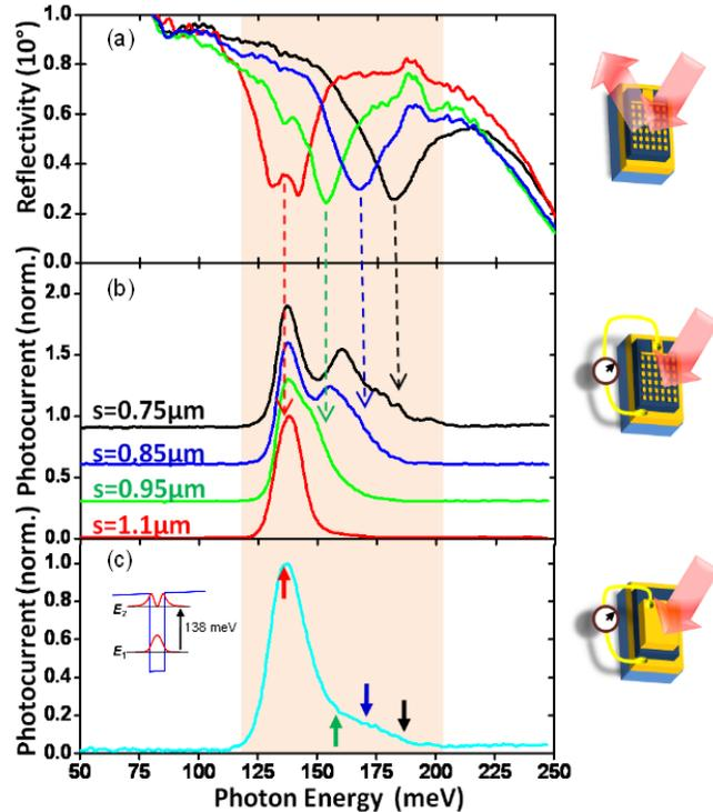
Fig. 2 (a) Reflectivity of the device of grating dimension  $s=0.75, 0.85, 0.95$  and  $1.1 \mu\text{m}$  at 77K. (b) Spectral photocurrent response of the devices. (c) Spectral photocurrent response of the double metal mesa of dimension  $200 \times 200 \mu\text{m}^2$ .
