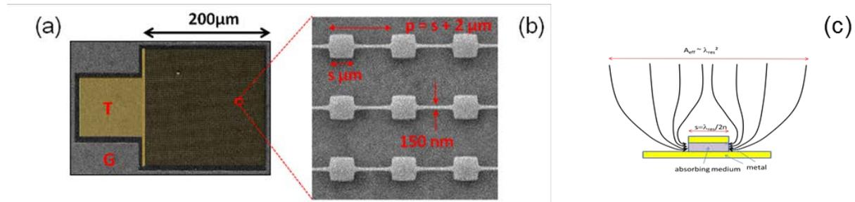
Fig. 1: (a) SEM picture of the device (top view). (b) Details of the subwavelength structure. (c) Schematic of the electric field harvested by the metallic patches on an area much bigger than the pixel surface.
