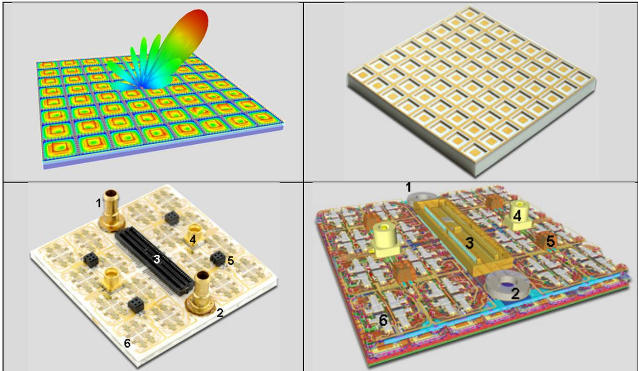
1: Liquid cooling inlet, 2: Liquid cooling outlet, 3: IF connector, 4: LO mini-SMP connector, 5: DC connector
