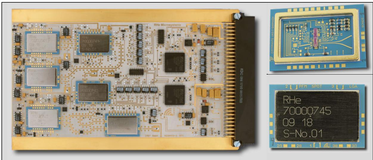
KERAMIS™ Technology: LTCC Modules for Satellite Communication in Ka-band
