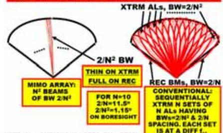
NOTE: AL=AMBIGUOUS LOBES; BM=BEAMS; BW=BEAMWIDTH; BWs GIVEN IN  $\omega$ -SPACE,  $\omega = \sin\theta$ ; L=CARRIER FREQ.
