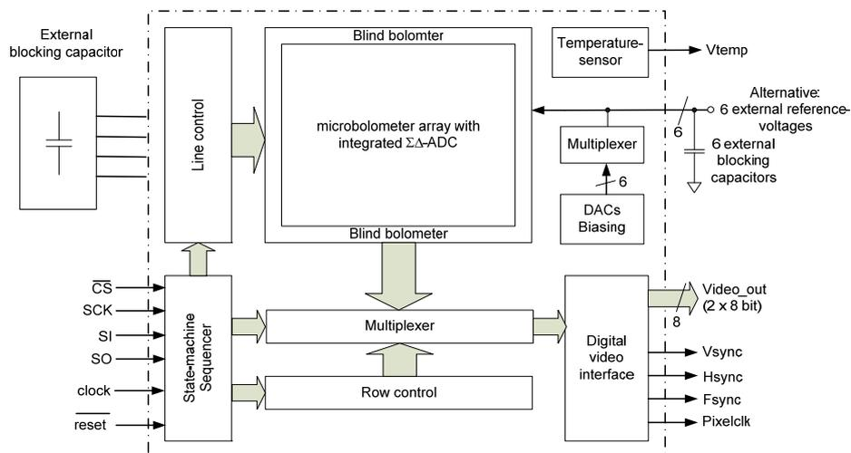
**Fig. 3** Block diagram ROIC of digital QVGA-IRFPA
