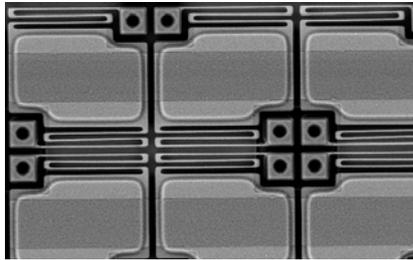
**Fig. 1** SEM micrograph of a bolometer (left: top view)
