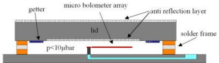
**Fig. 2** Principle of a chip-scale vacuum package
