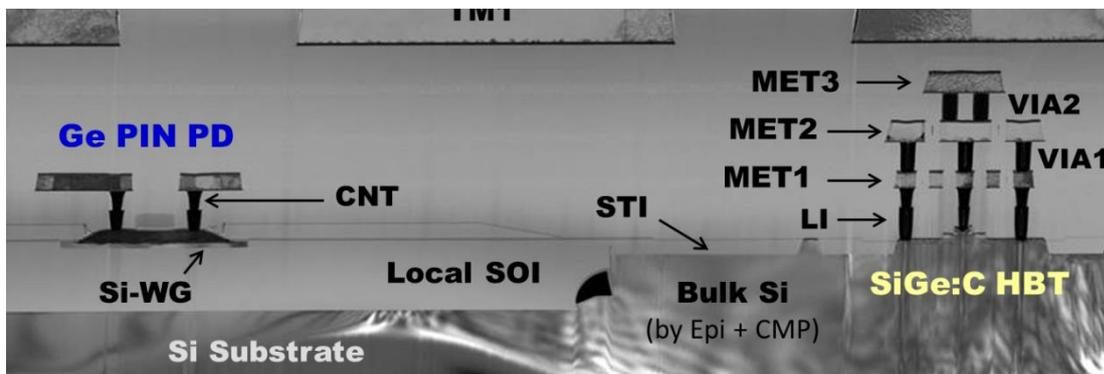
Figure 3: Cross section of photonic SiGe-BiCMOS technology components including Ge-photo detectors (left) and HBT devices (right) with peak cutoff-frequencies ( $f_T$ ) and maximum oscillation frequencies ( $f_{max}$ ) of 190 GHz at  $BV_{CE0}$  of 1.9V. [3]
