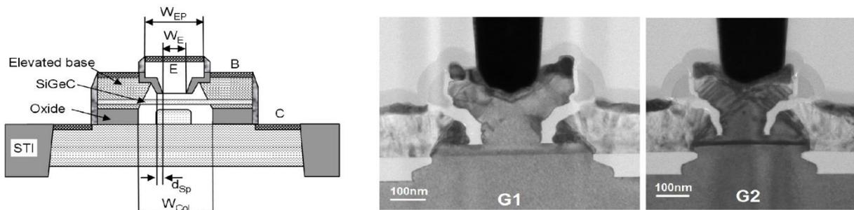
Figure 2: Schematic (left) and silicon processed (right) cross section of two types of high performance SiGe-HBTs featuring devices with peak cutoff-frequencies ( $f_T$ ) and maximum oscillation frequencies ( $f_{max}$ ) of 300 and 500 GHz can be achieved at  $BV_{CE0}$  of 1.7V. [2]
