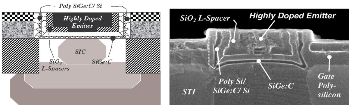
Figure 1: Schematic (left) and silicon processed (right) cross section of a SiGe-HBT realized by only one additional mask to the underlying CMOS process. Peak cutoff-frequencies ( $f_T$ ) and maximum oscillation frequencies ( $f_{max}$ ) of 90 and 75 GHz can be achieved at  $BV_{CE0}$  of 2.4V [1].
