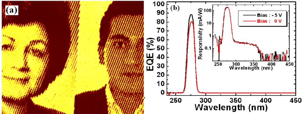
Figure 3. (a)  $320 \times 256$  UV image. (b) Photodetector (PD) showed unbiased peak responsivity of  $\sim 176$  mA/W, increasing to  $\sim 192$  mA/W under 5 volts of reverse bias.
