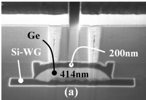
Fig. 1: SEM cross-sections of a Ge photodiode fabricated in a BiCMOS compatible process flow [8].
