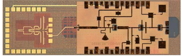
Fig. 3: Chip photo of the heterogeneous integrated signal source at 164 GHz. VCO in BiCMOS and doubler-amplifier combination in InP [10].
